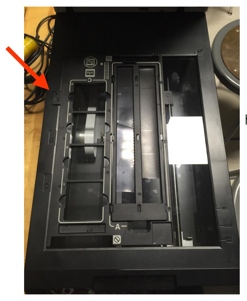
2. Place negative holder in scanner bed, matching the "A" tab with the "A" on the scanner bed.
